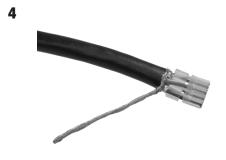
Slide the load bar/liner all the way down flush to the pair spacer bar and trim conductors flush against the load bar/liner front end using the 5" Side cutting Pliers, P/N 10531C.
