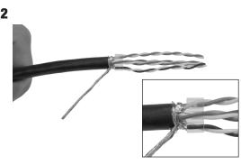
Using supplied pair spacer bar, insert pair 1-2 through left box, pair 7-8 through right box, and place pair 5-4 in top groove, pair 3-6 in bottom groove. Orientation will depend on your wiring sequence. Make sure spacer bar is placed next to cable jacket.
