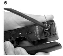
Insert connector into the Tele-Titan XG 2.0 crimp tool and compress the handle. The contacts are terminated.
